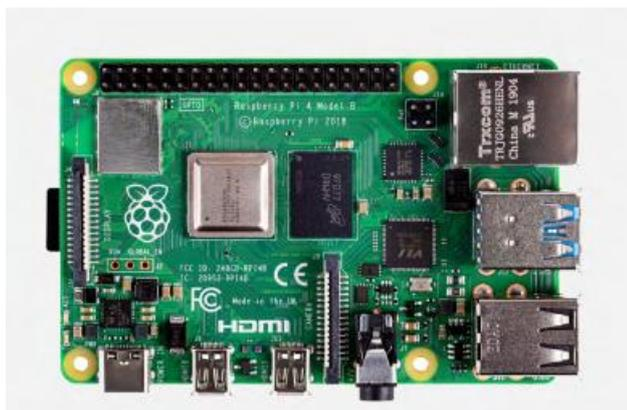
Figura 13 - Raspberry Pi 4 - Model B. Fonte: Raspberry Pi website.
