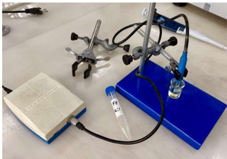
Figura 14 – Montagem experimental. (a) \mu Stat 400; (b) PGSTAT302N.
