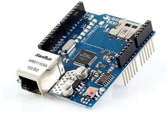
**Figura 18: Shield Ethernet [16].**
